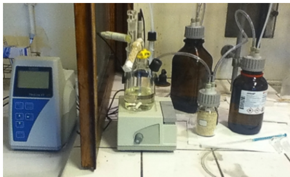
FIGURE 2.9: A Karl Fischer apparatus. All its components are connected to a desiccating material in order to prevent humidity intake from influencing the measurements.
