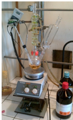
FIGURE 2.6: Typical apparatus used for the synthesis of Cho-AA ionic liquids.
