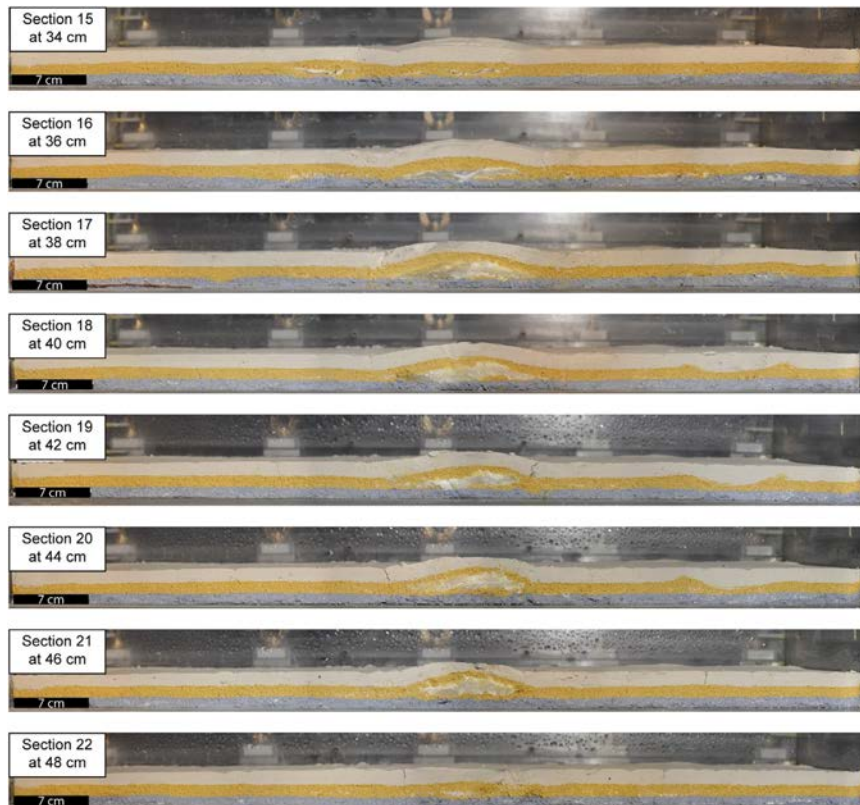
Figure 4. Selection of 8 full-length serial cross-sections, Experiment 4 – Series II (no applied horizontal deformation). For number and position of each section, see key (top left). Wax has migrated upward (and laterally) through pore space, from basal blue source layer and into open horizontal hydraulic fractures, forming sills (white) upon solidifying. At centre of model, sills are most numerous and thick within yellow layer; whereas, near edges of model, some sills are visible in blue basal source layer. Large bulges at top of model are above thick sills within source layers. Scale bar is 7 cm long. (For interpretation of the references to colour in this figure legend, the reader is referred to the web version of this article.)
