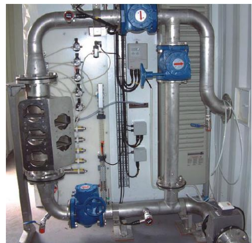
Fig 1.6: Configurations of (a) Ultrawaves and (b) Sonix™ reactor
