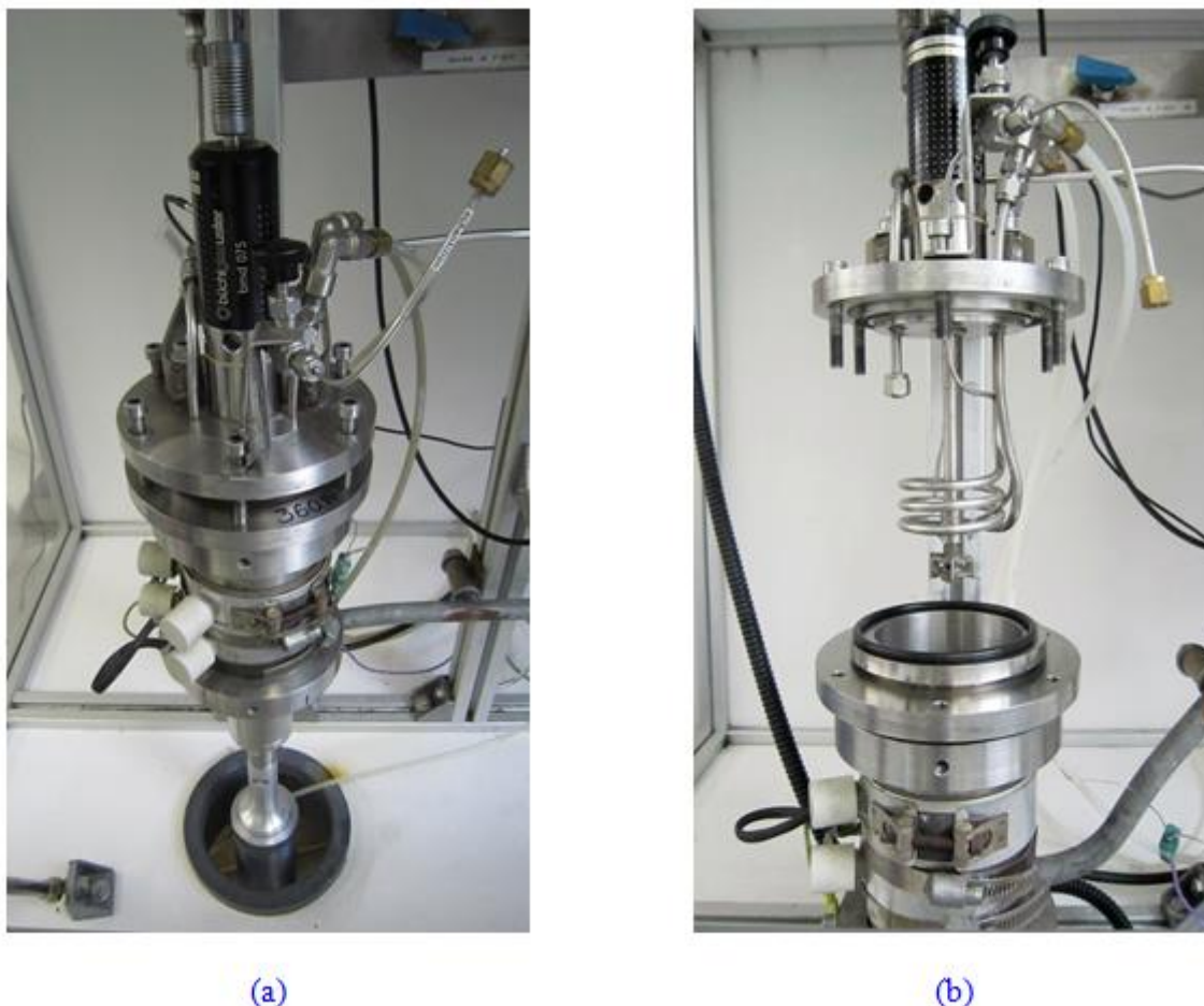
Fig 2.5: (a) Closed and (b) opened cup-horn autoclave reactor
