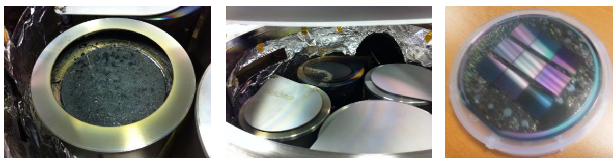
Fig. 57a: illustrations of sputtering machine pollution issues encountered on the silica target (left) and over the covers (middle) due to flaking phenomenon and a long absence of vacuum, and impact on a wafer after 120 minutes silica sputtering (right).
