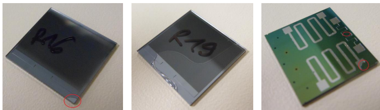
Fig. 57b: illustrations of fabrication issues encountered: benign irregularity (left) and serious default (middle) of Pyrex bonding, and platinum filaments partial tearing (right).
