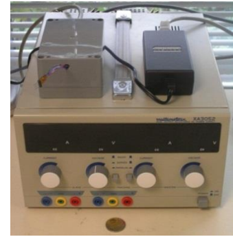
Fig. 60c: power supplies (OA, fans, heater + Peltier)
