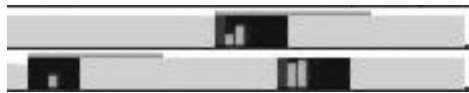
Figure 2: First type of inconsistency. The horizontal axis is the time (in weeks) and each line on the vertical axis corresponds to a power plant. Outages are represented by black rectangles and production level are in gray. Inside an outage the first bar represents the level of fuel added during the outage, the second and third ones correspond to the bound on the fuel level. The rightmost outage may be removed from the solution by adding more fuel in the previous outage.
