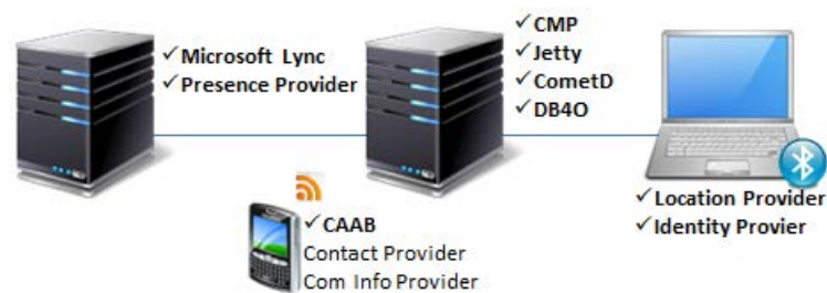
Figure 6.2: CAAB deployment architecture
