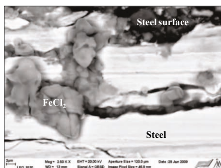
Figure 22. BSE-SEM image of the cross-section of the 10CrMo9-10 steel ring after 7 h with doped fuel and a test ring temperature of 450 °C (Paper IV).
