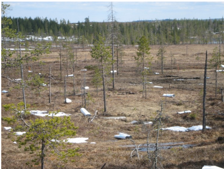
Figure 4. Target units were positioned in lines. The distance between adjacent target dummies was 10 meters.
