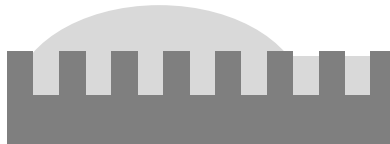
Figure 4. A liquid film is formed ahead of the droplet, when the contact angle is between 0 and a critical value \theta_C .
