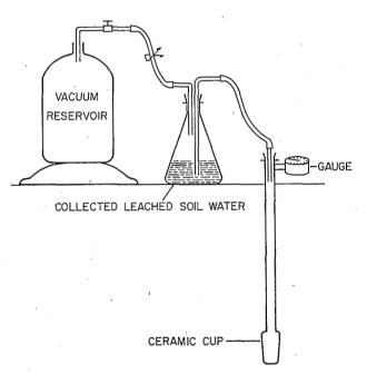
Fig. 2. Diagram of the field system used for collecting aldicarb in the subsurface soil water to a depth of 61 cm.
