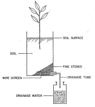
Fig. 1. Diagram of greenhouse pot system used for collecting aldicarb in soil leachates.
