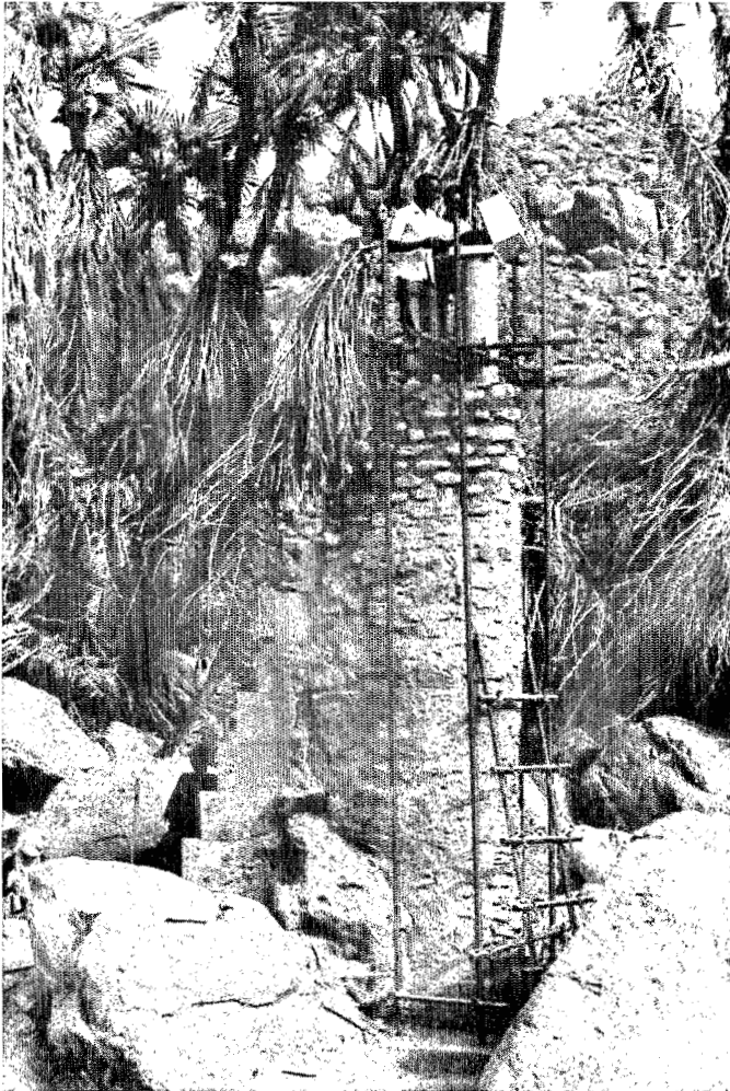
Figure 13.8 Water level recorder at Adoubdoub on Tamgak (representative basin), (Air, Niger Republic)
