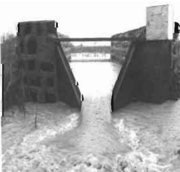
This H-flume measures runoff from an area of cultivated Vertisols.
