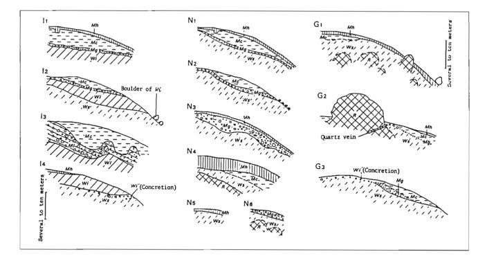
Figure 6 : Regolith-profile types and their series (adapted from Tamura, 1986a). See the text and figure 5 for abreviation.
