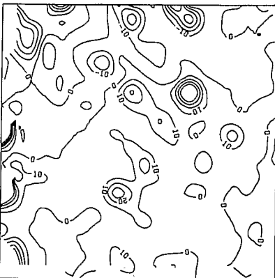
Fig. 6. Residuals obtained by polynomial interpolation from profile distribution of points. The only difference between (a) (top) and (b) is the spacing of profiles which is wider in (b).
