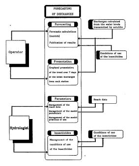
Fig. 5. Flow diagram of the forecasting part of the PERLES software.
