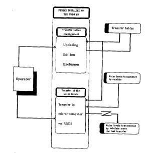
Fig. 3. Flow diagram of the PERLES software at the data reception station.
