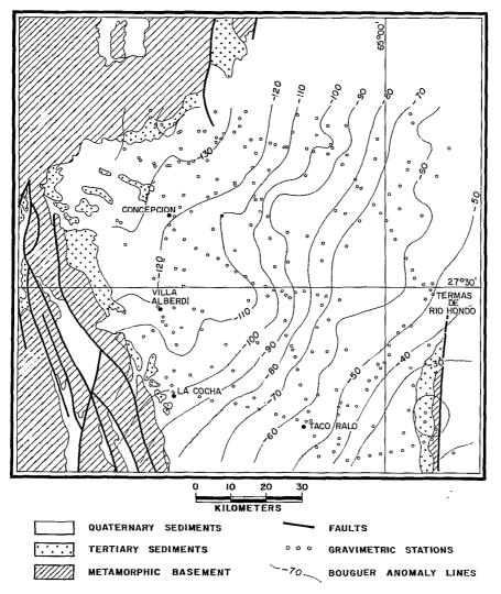
Fig. 2. — Geological map of the Tucumán Basin, Bouguer anomaly field contoured at 10 mgal intervals and the distribution of the gravity stations.
