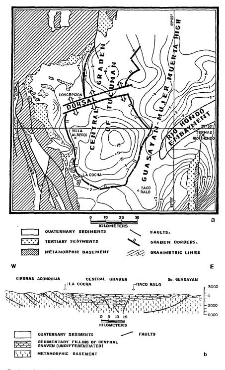
Fig. 3. — Geological map of the Tucumán Basin a - Residual anomaly field contoured at 4 mgal. b - The qualitative model.
