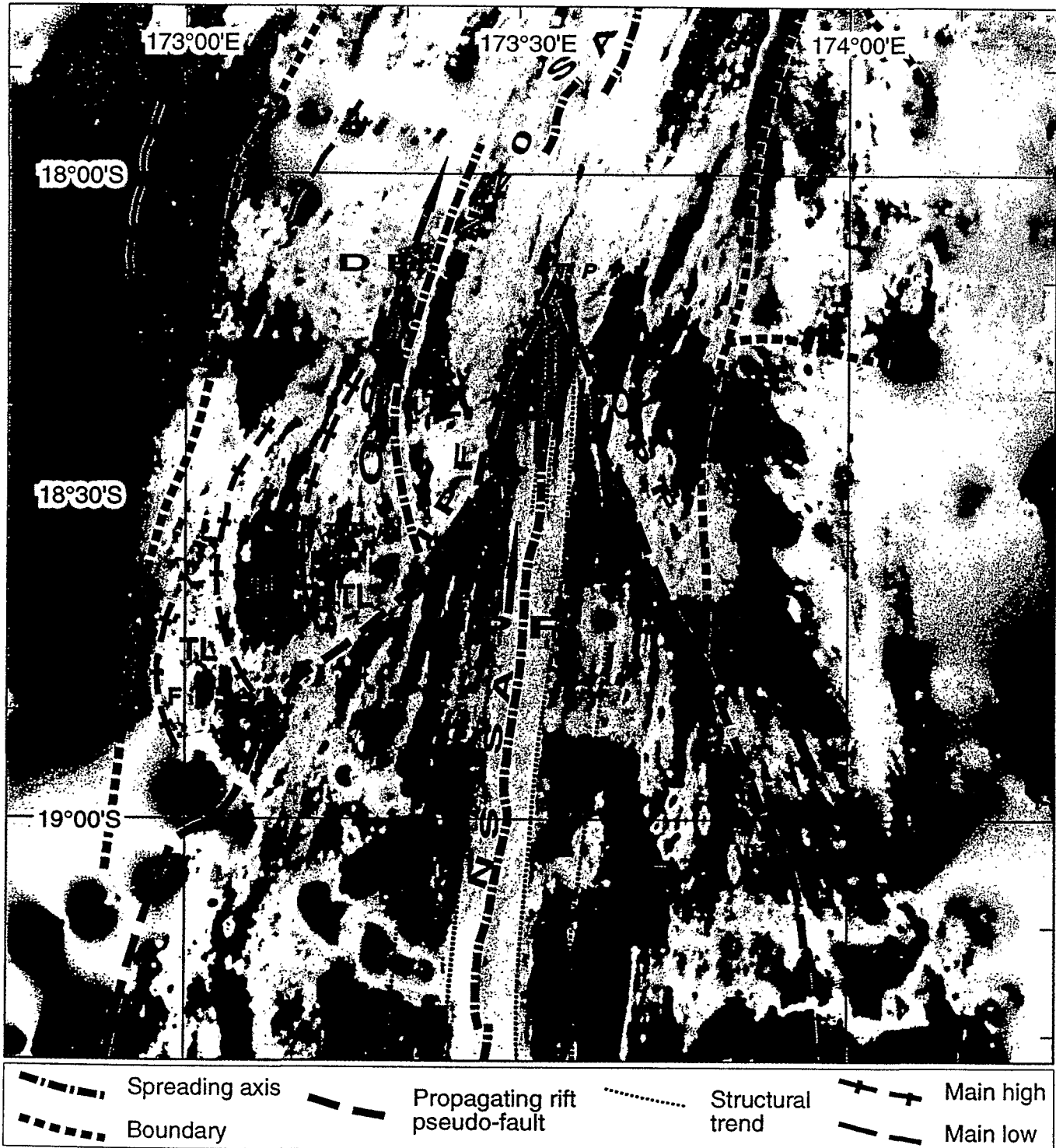
Fig. 10. Tectonic pattern matched with the digital elevation model (DEM) of the propagating rift (Ifo-Khoros-Istar processing). DR =dying rift; FR =failed rift; IPF =inner pseudo-fault; N20 SA =N20°E spreading axis; NS SA =N-S spreading axis; OPF =outer pseudo-fault; OSC =overlapping spreading center; PR =propagating rift; TDR =active tip of the dying rift; TL =transferred lithosphere; TPR =tip of the propagating rift; TZ =transform zone.
