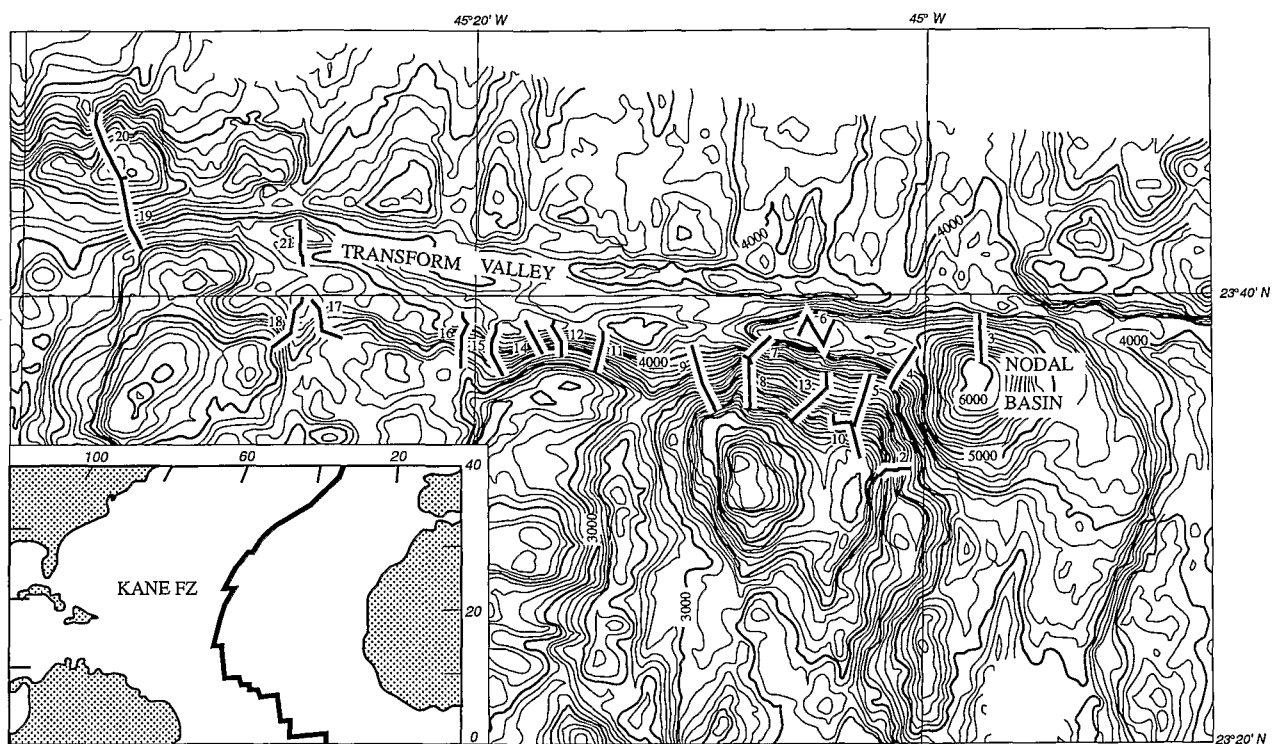
Fig. 1. (a) Location of the Kane FZ in the Central Atlantic. (b) Multibeam Bathymetry of the Eastern half of the Kane FZ. The contour interval is 100 m. The dives tracks are in heavy lines.
