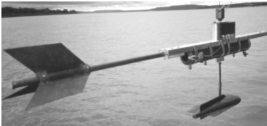
Fig.2. The HiBAM punctual sampler built from an oceanographic bottle, with a 12 litres of nominal volume adapted to be used in big rivers.
