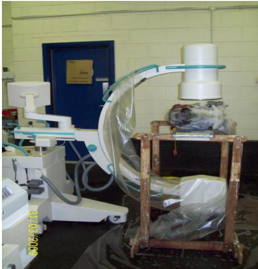
Figure 2-2: Setup of fluoroscopic machine and the specimen.
