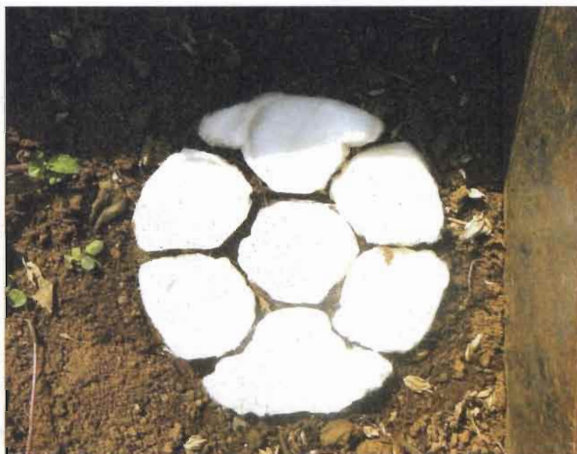
Figure 7 – Wet cotton wool after infiltrometer use and tube guide removal. Note the well separated infiltration zones.
