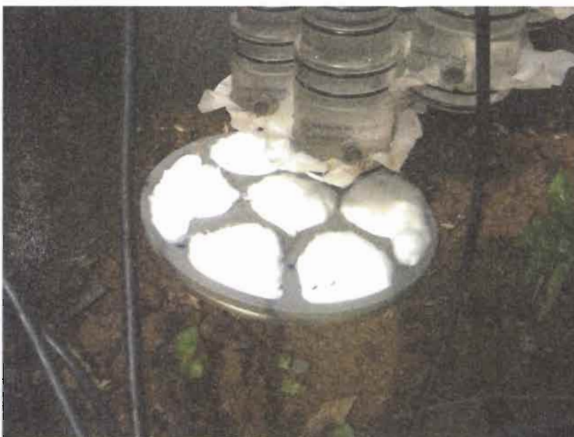
Figure 3 – Cotton wool ensuring contact between the infiltrating tubes and soil
