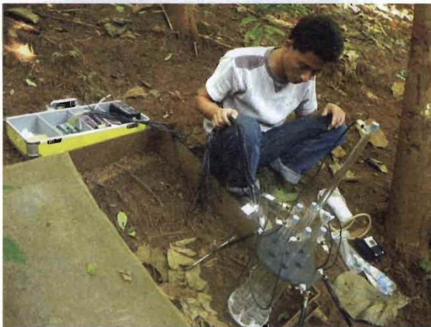
Figure 5 – The new infiltrrometer with tripod on a 67.5% slope.
