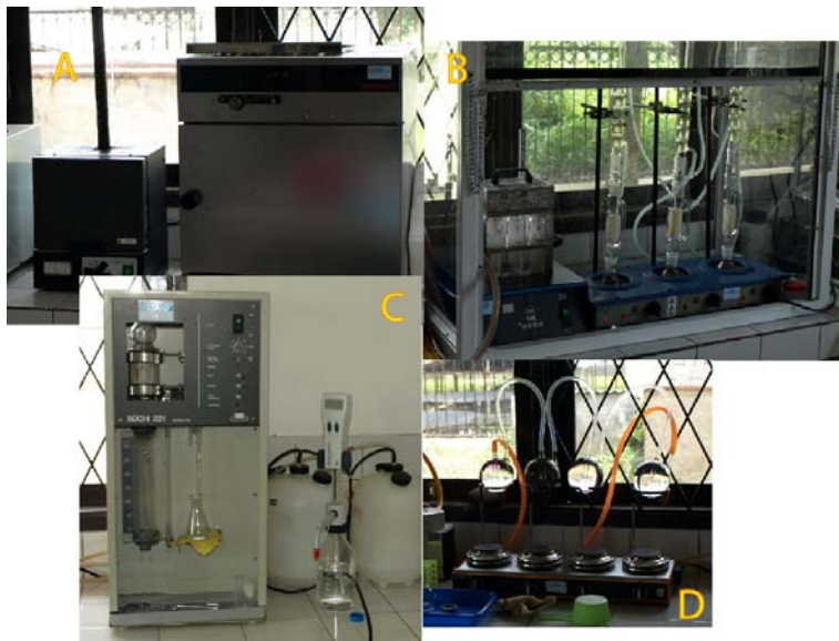
Figure 21 Equipment newly available in Depok laboratory for determination of proximate analysis: Oven and furnace (A), Kjeldahl mineralization and Soxhlet extraction (B), Kjeldahl distillation and titration (C), and crude fiber analysis (D)
