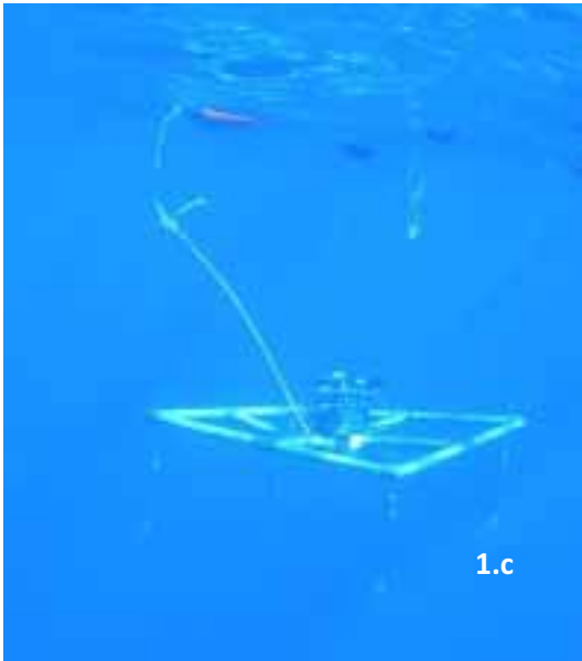
Fig. 1.c & 1.d: PVC frame equipped with a camcorder, 4 branchlines and 4 buoys
