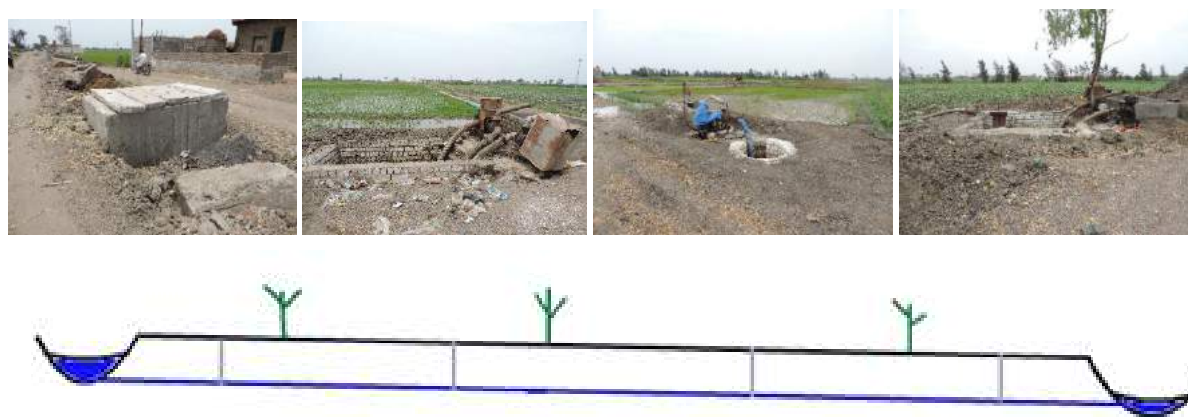
Figure 13. Deep piped-systems from intake point near canal, individual pits, to outlet gate at drain
