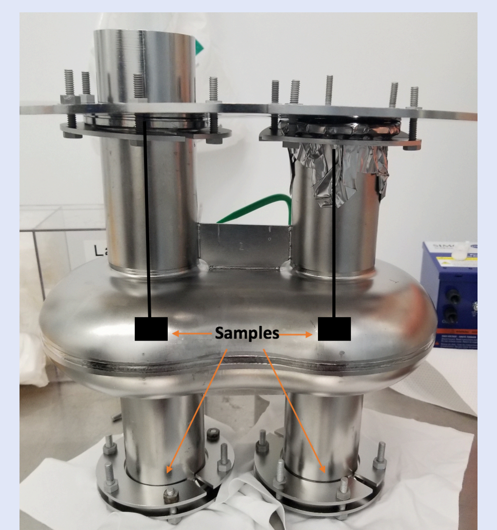
Cavity assembly for coating.
