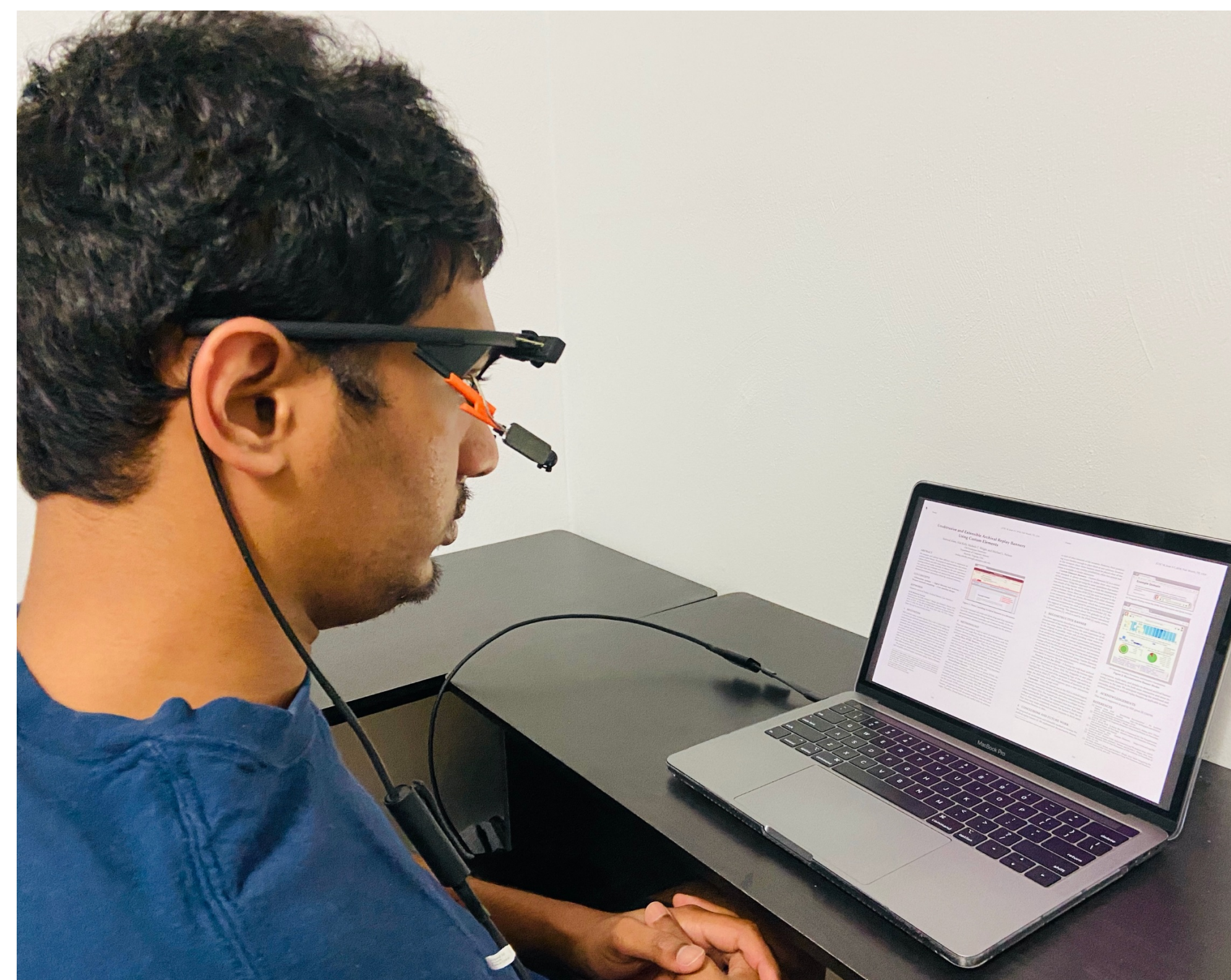
Fig 1. A participant reading the research paper while wearing the PupilLabs Core eye tracker
