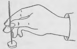
Fig. 117. DRILLING WITH BRISTLE.
