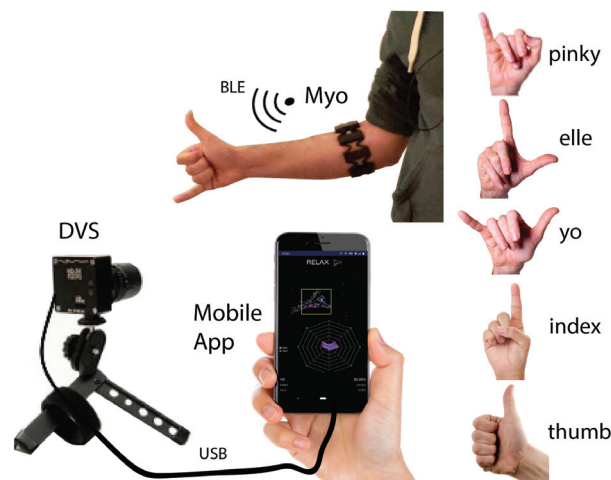
Fig. 1: On the left, the demonstration setup: Myo on the subject forearm, DVS looking at the gesture and mobile application. On the right, the five gestures of the classification.
