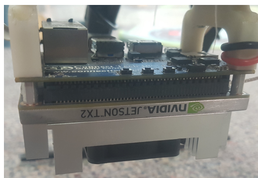
Figure 3.6: NVIDIA Tegra TX2 connected to the compact ConnectTech Orbitty Carrier Board
