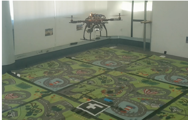
Figure 5.2: Quadrotor Experiment with assistance of the ArUco marker
