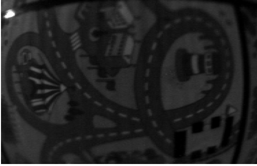
Figure 4.5: Semi-textured surface raw image. From a hovering quadrotor with a downwards facing camera while computing optical flow.
