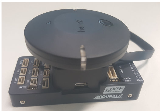
Figure 3.5: Pixhawk 2.1 with HERE2 GNSS mounted on top
