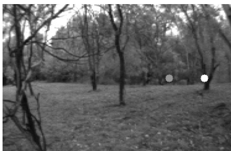
Figure 6.10: Raw image output of the mvBlueFOX-200w camera at a resolution of 376x240. The grey dot is the vector {}^A\hat{v} plotted on the camera frame, while the white dot is the desired velocity vector determined from \epsilon .
