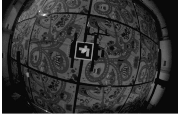
Figure 5.1: ArUco Marker Detection. The grey dot in the centre of the ArUco fiducial marker is the calculated centre of the ArUco marker using the marker corners.
