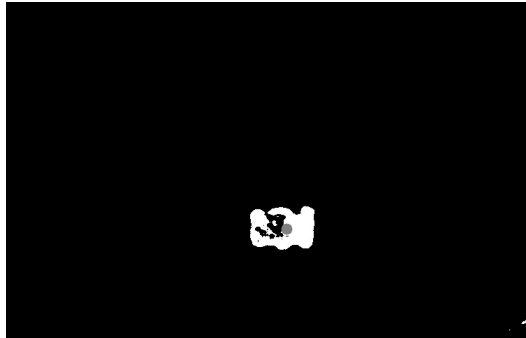
Figure 5.8: Colour Segmented Output. The grey dot in the centre of the white area is the calculated centre of the coloured target.
