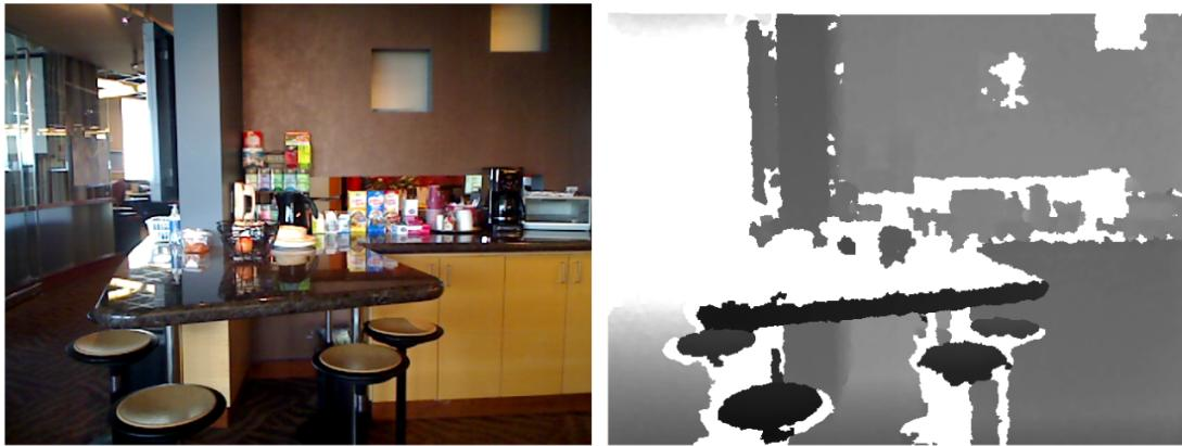
Figure 1.6: Illustration of RGB image (left) and depth (right) information captured by an RGB-D camera. (source: [Henry et al., 2014])
