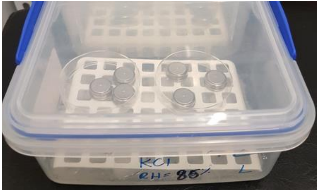
Figure 4-2 Calibration of humidity sensors of I-buttons in potassium chloride solution at 20 °C.
