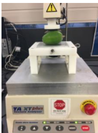
Figure 3-1 Compression firmness measurement of feijoa.
