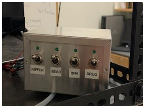
Figure 22: Custom designed flow control box to flow our four biomaterials. Upon flipping of a single switch, it will induce the solenoid (not shown) to move a magnetic clamp allowing for compressed air to flow through the tubing to the reservoir holders at adjustable pressure.
