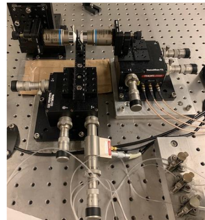
Figure 24: The stage (front) that is used to mount the flow-cell. The two shorter length knobs (coming towards the front and left) are for manual control and the longer knob coming towards the front can be manipulated both manually and by the computer.
