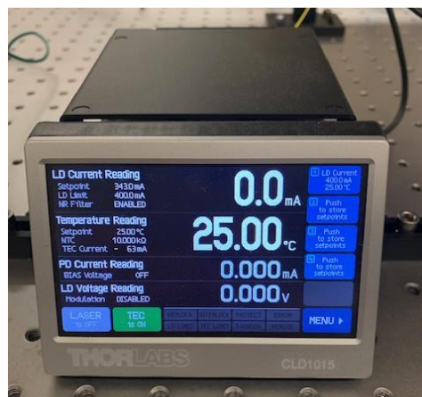
Figure 26: Laser controller that houses the laser that is used for the optical tweezers.
