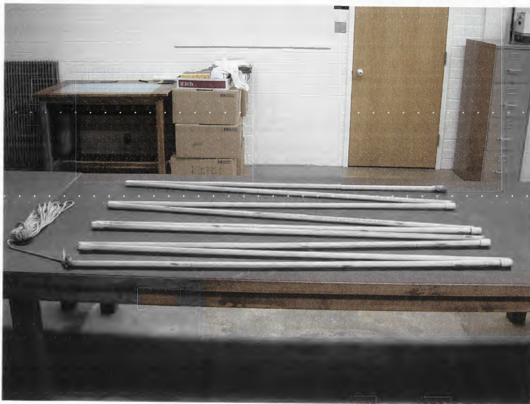
Fig. 3.39 Photograph showing the interconnectable PVC pipes used to push the horizontal inclinometer into the H2 casing
