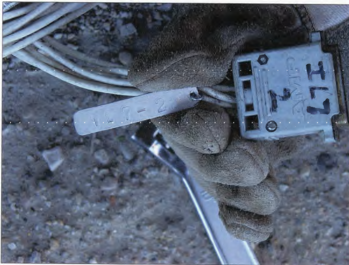
Fig. 3.18 Aluminum tags used to label the strain gage connectors
