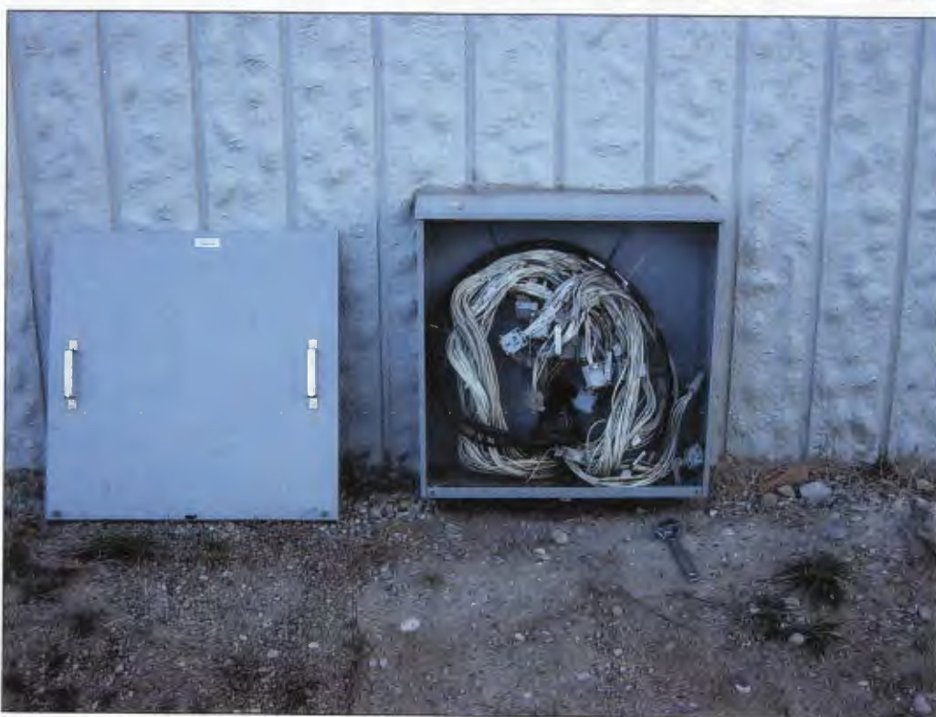
Fig. 3.20 Close up views of the north box containing strain gage cables and connectors
