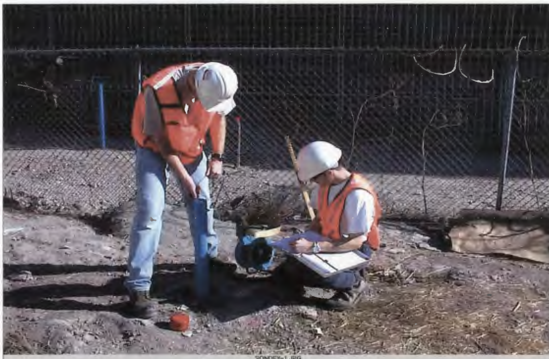
Fig. 3.15 Photographs showing Sondex sensor and readings being taken in the field
