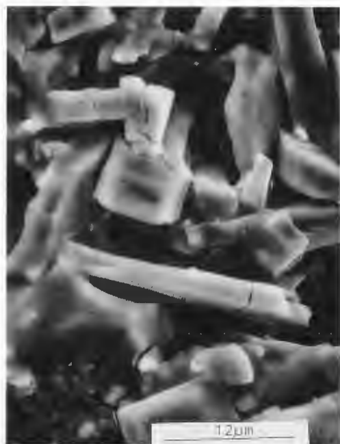
Fig. 12: Microstructure after 1 hr. at 760°C
