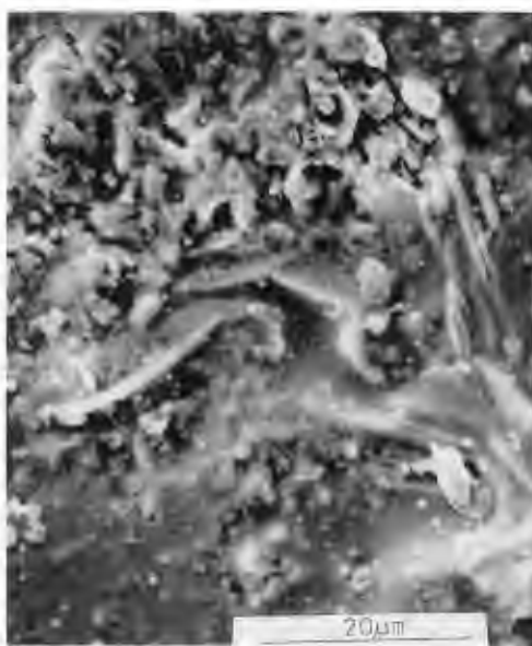
Fig. 11: Microstructure after 1 hr. at 705°C
