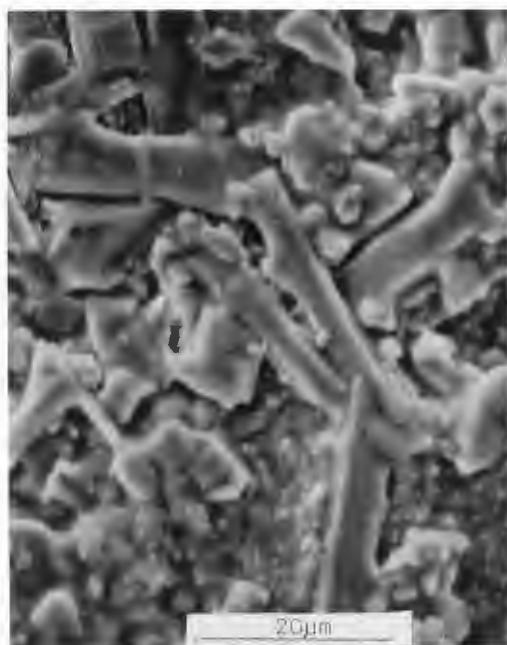
Fig. 14: Microstructure after 1 hr. at 870°C
