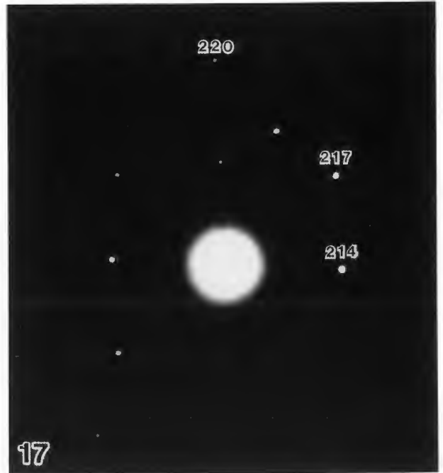
Fig. 17. Electron diffraction pattern of whitlockite in a rhombohedrally based crystal similar to those of Figure 14. The [214], [217], and [220] planes are clearly seen.
