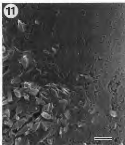
Figure 8. SEM image of acicular crystalloids with columnar crystals around them. Bar = 1 \mu\text{m} .
