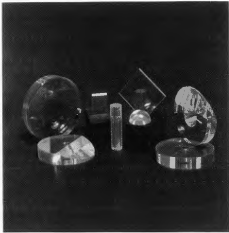
Fig. 11. Single crystal scintillators for BSE detectors.
