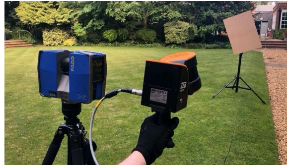
Figure 1: Scanning a target using static (on the left) and mobile (in the middle) laser scanners.
