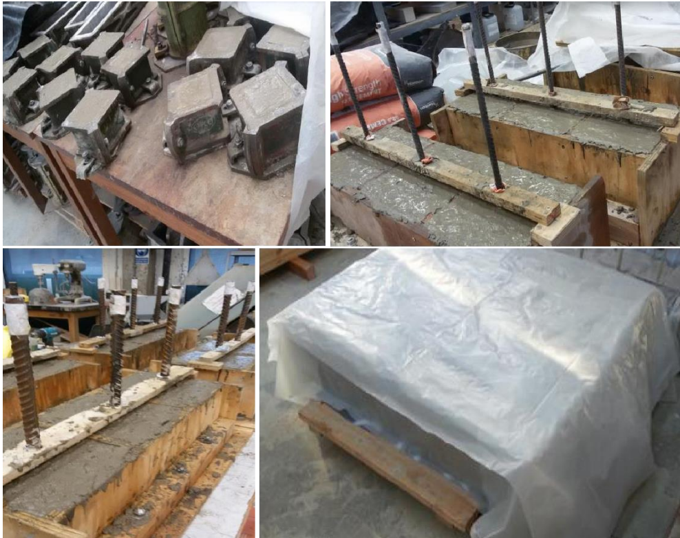
Figure 3. 4 Casting and curing pull-out specimens.
