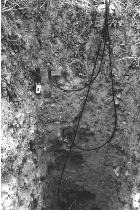
Plate 7: Soil profile developed in weathered marl with installed TDR-sensors
