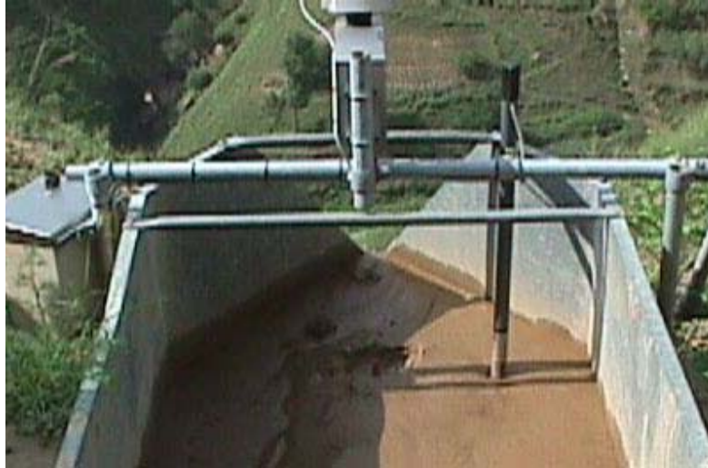
Figure 5.5 Thick sediment layer (about 10 cm) in the gully-flume after the event of 980712. At this time the barrels below the flume had not yet been installed. Picture by E. van de Giessen and J. Snepvangers
