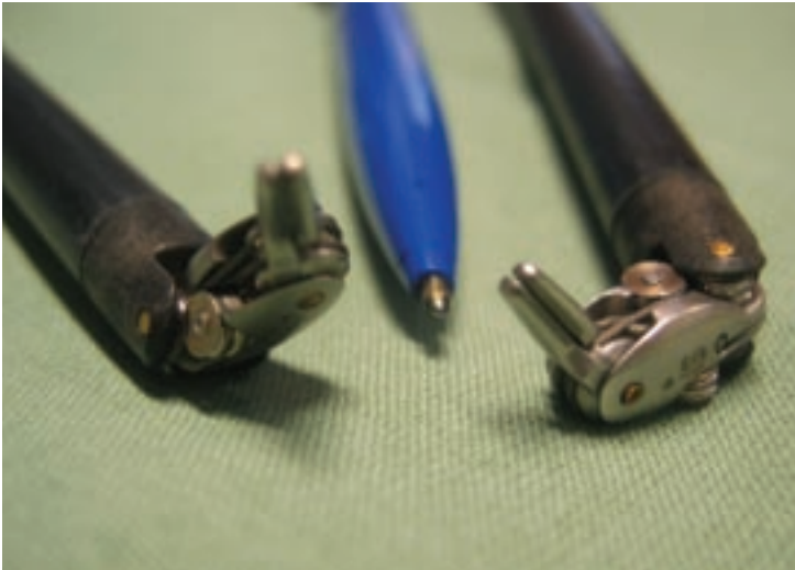
Figure 10 The da Vinci instruments provide two additional degrees of freedom at the tip of the instrument.
