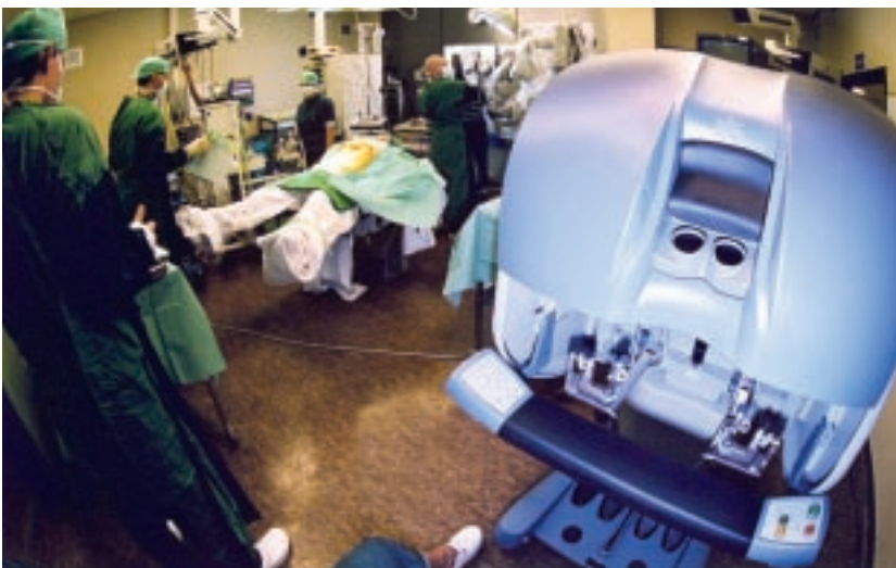
Figure 3 The console integrates two manipulators, placed in line with the 3-D display of the surgical field.
