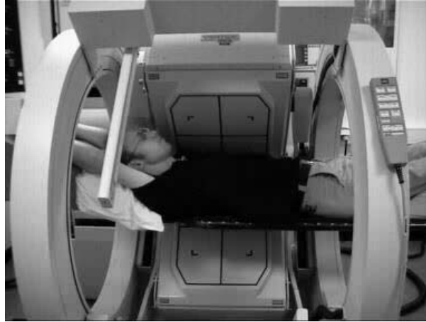
Figure 1.3: Example of an ECT-TCT system. This system uses two scanning line sources containing Gadolinium to acquire the transmission data.
