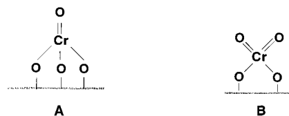
Figure 1. Molecular structure of a supported monochromate species: (a) mono-oxo species and (b) di-oxo species.
