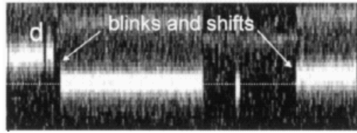
Figure 10: Correlation between blinking of a CdSe/ZnS nanocrystal (measured at 10 K and using \lambda_{\text{ex}} = 514 \text{ nm} ) and a shift in the average emission wavelength. Data taken from Ref. [32] with kind permission from the authors.
