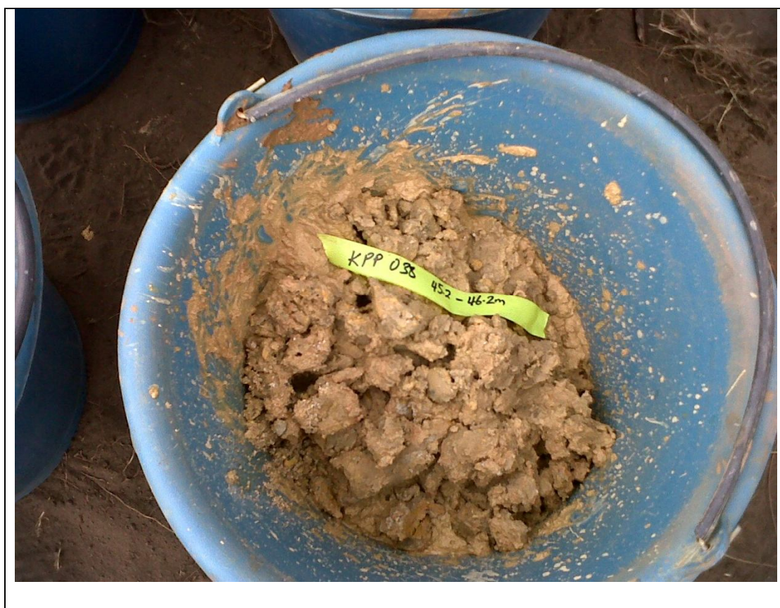
Figure 3.7_1: A photo showing the blue bucket with a phosphate sample recovered by Aircore drilling technique. A yellow tag with sample identification number is also shown.
