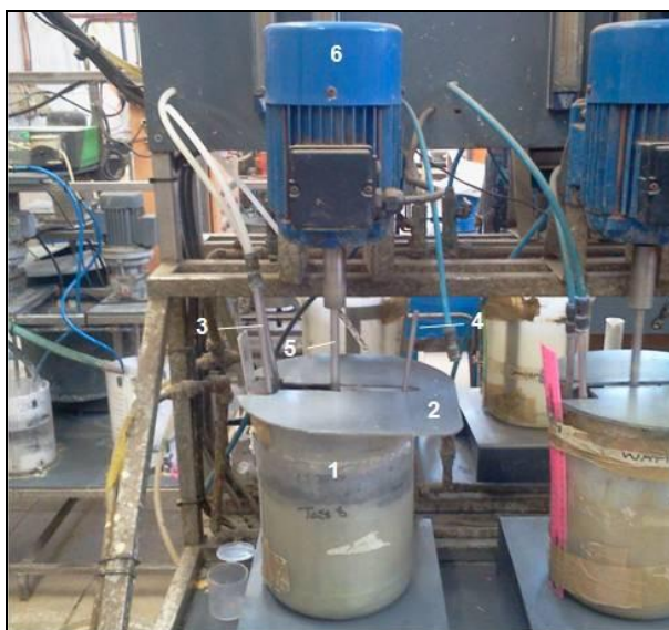
Figure 55: Batch reactor used in the leach tests. The tests were conducted in 5 L plastic beakers (1), with Perspex covers to limit evaporation (2). Temperature was controlled by circulating warm water through a stainless steel loop (3). The reactor had the facility (not used in the present study) to introduce gas into the reaction through a stainless steel tube (4). Agitation was achieved by a four blade impellor (5) rotated by an electric motor (6).
