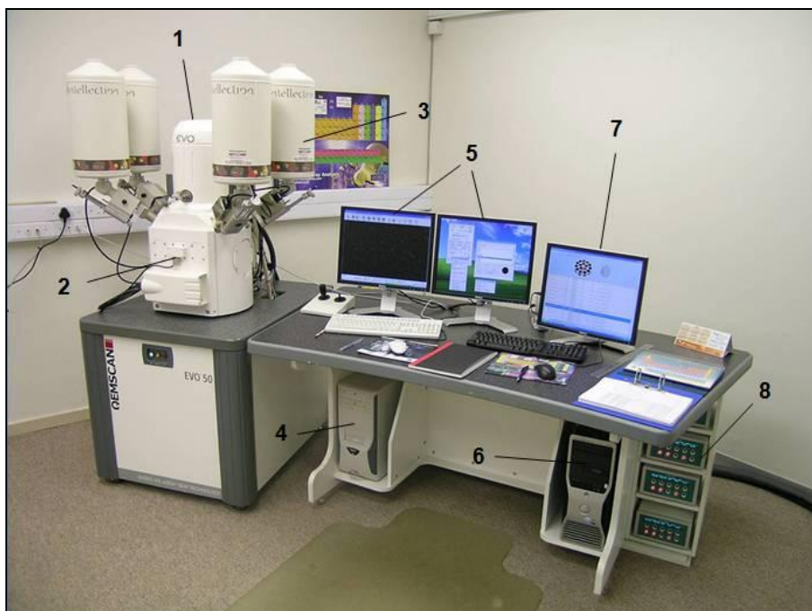
Figure 35: One of the QEMSCANS at SGS South Africa, showing the electron gun and column (1), the chamber into which the samples are loaded (2), the energy dispersive X-ray detectors (3), the standard Evo 50 computer (4) with its two monitors (5), the additional computer providing QEMSCAN capacity (6), with its monitor (7) and the pulse processors (8) which convert the signal from the X-ray detectors into a signal that the computer can process.
