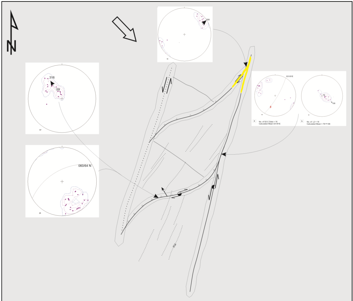
Figure 6.18: The schematic summary of the overall tectonics during D2 deformation, depicting the structures that were reactivated or formed during D2 deformation. The tectonic transport direction in D2 was towards the southwest. Yellow lines are indicating the mylonite zone.
