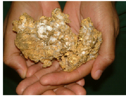
Fig. 4: 1.217 Kg nugget of gold-quartz from 18m depth in the Essakane ore deposit (Anon, 2008).
