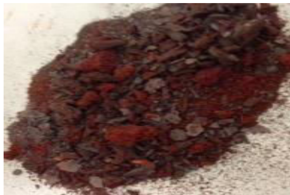
Figure 4.12: Leaching residue containing iron(III) acetylacetonate crystals
