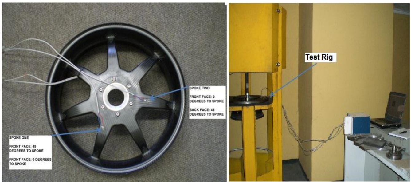
Figure 9: Strain Gauged Ducati Rim and Experimental Setup [edited 8]
